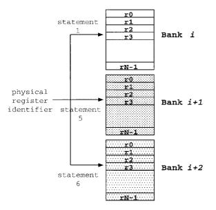
Fig. 3 Bank-based register file.
