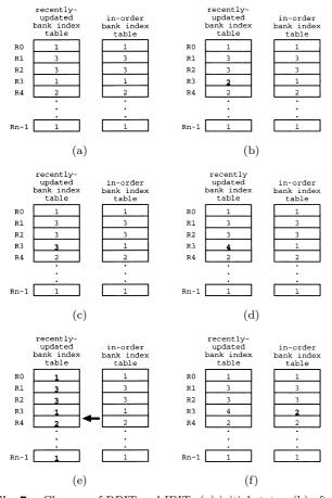
Fig. 7 Changes of RBIT and IBIT. (a) initial states, (b) after issue order 1 is issued, (c) after issue order 5 is issued, (d) after issue order 6 is issued, (e) interrupt handling when an interrupt occurs at (c) or (d), (e) after issue order 1 is completed without exception.
